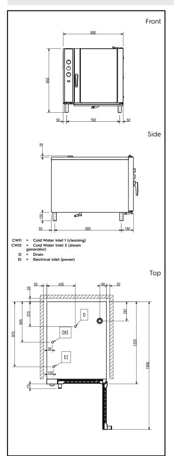
**Electric** Supply voltage: 380-400 V/3N ph/50 Hz Auxiliary: 0.5 kW Electrical power max: 24.5 kW Capacity: Trays type: 10 (GN 2/1) **Key Information:** External dimensions, Width: 890 mm External dimensions, Depth: 1215 mm External dimensions, Height: 970 mm Net weight: 147 kg Height adjustment: 80/0 mm Functional level: Basic Cooking cycles - air-convection: 300 °C
